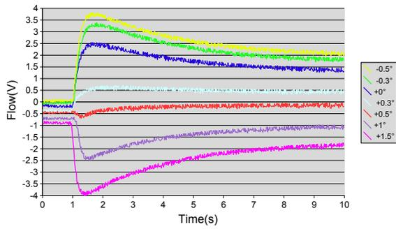
Fig. 3. TEM flow evolution. Temperatures are relative to ambient air
