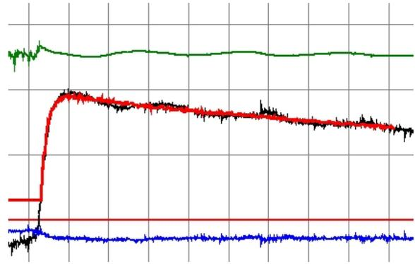
Fig. 5. Flow tracking of metal (in red:desired, in black:obtained, in green:current control)
