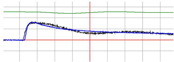
Fig. 6. Flow tracking of wood (in blue:desired, in black:obtained, in green:current control)
